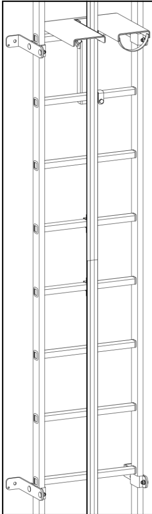
Aluminium access ladder rail profile 72 x 25 mm
