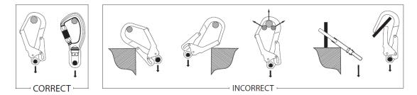
• It is necessary to protect the snap hook gate with locking gear. - See drawing.
