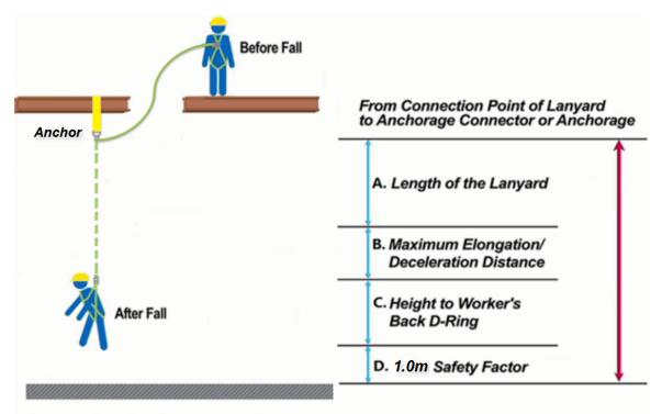
Minimum Free Fall Distance = 6.55m (Height to worker's back D-ring, usually 1.8 meters)
